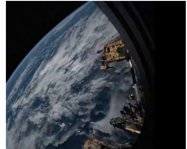
Figure 54: The SESAME module (highlighted in red circle) mounted on the ISS © ESA/NASA
